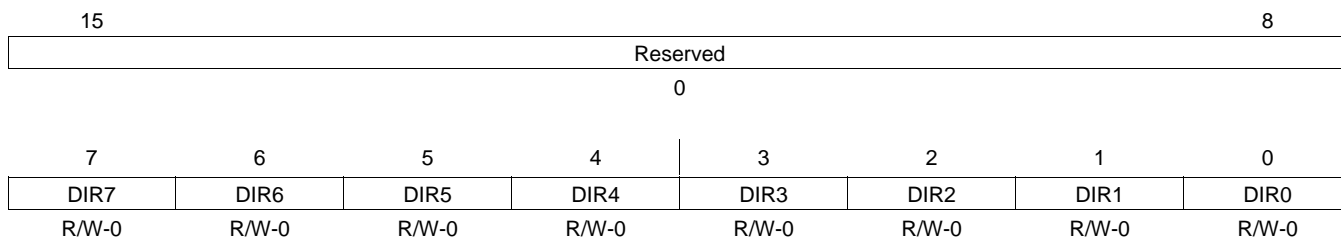
Figure 3-23. General-Purpose I/O Control Register (GPIOCR) [MMR Address 003Ch]
