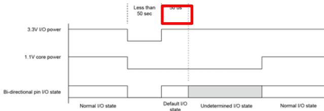
Figure Error! No text of specified style in document.-13 Timing Sequence with Undetermined I/O State
