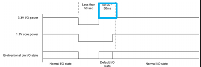
Figure Error! No text of specified style in document.-16 Recommended Power Sequence
