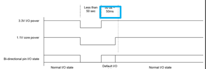
Figure Error! No text of specified style in document.-12 Recommended Power Sequence
