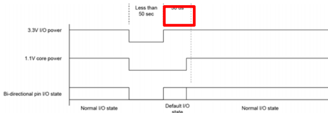
Figure Error! No text of specified style in document.-14 Recommended Power Sequence
