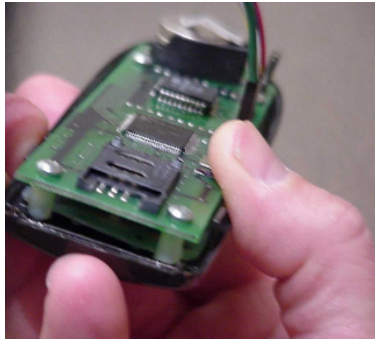
Figure 4: Care When Disconnecting JTAG
